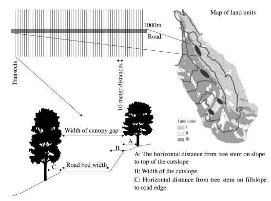
Figure 2. Sampling design for clearing limit of road in environmental units
