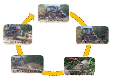
Figure 3. Main work elements in a cycle during winching operation with tractor
