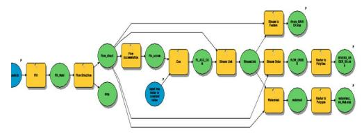
Figure 16. Hydrological analysis model
