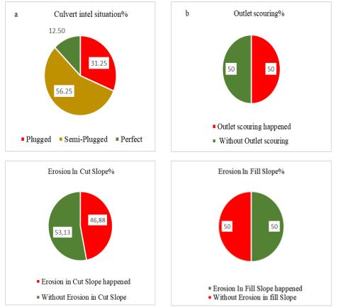
Figure 6. a) Intel situation in pipes, b) Outlet scouring in pipes, c) occurred erosion in culvert's cut slopes, d) the erosion taken place in pipe's fill slopes
