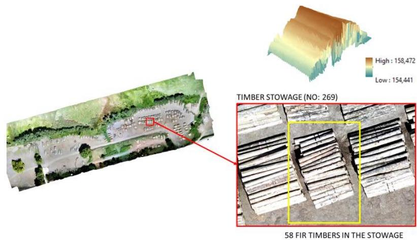
Figure 9. Timber stowage (No: 269) used for volume comparison
