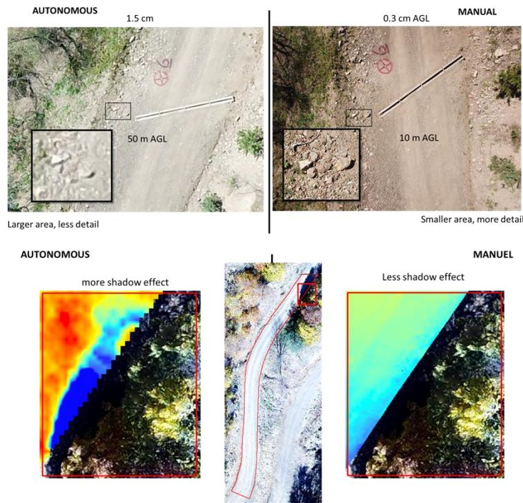
Figure 8. Comparison of autonomous and manual flights in terms of shadow effect (bottom) and object details in the images
