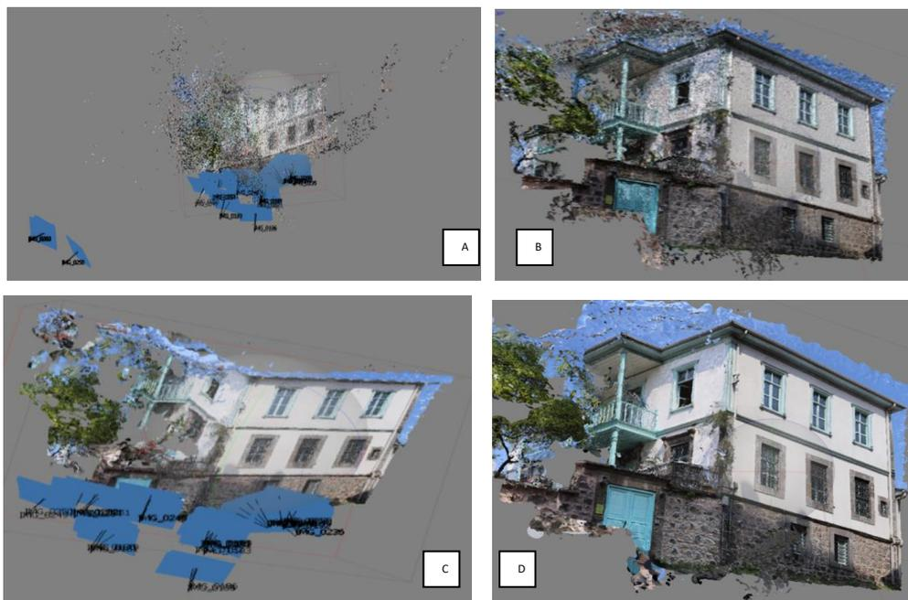
Figure 3. A) Tie points view of the house with camera positions, B) Dense Point cloud view of the house, C) 3D Model of the house with camera positions, and D) 3D Model view of traditional house
