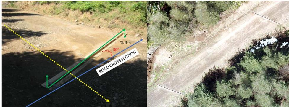
Figure 3. The open-top culverts are installed over the road surface
