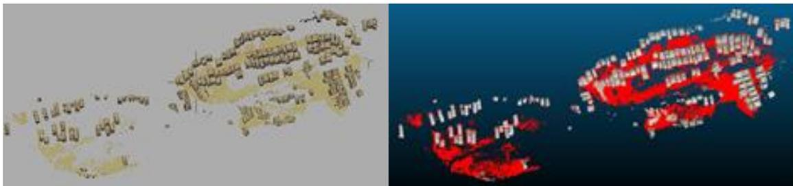
Figure 3. Dense point cloud filtered (left) and refined cloud (right)
