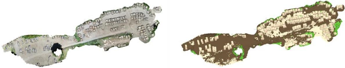
Figure 2. Dense point cloud (left) and dense point cloud classified into three classes such as ground (brown), high-vegetation (green), and man-made (corresponding to timber stowage) (white) (right)
