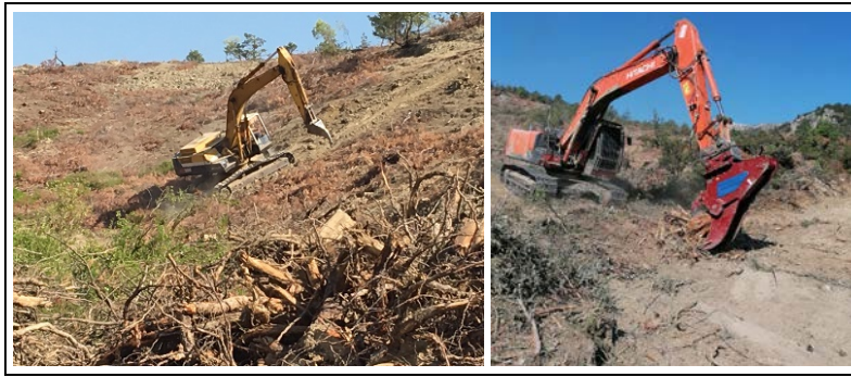
Figure 5. Excavator attachments for stump harvest: Ripper (at left) and Splitter/shear (at right)
