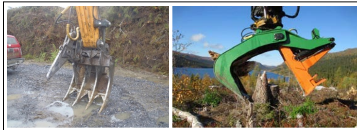
Figure 11. Excavator attachments as a splitter in different countries for stump uprooting
