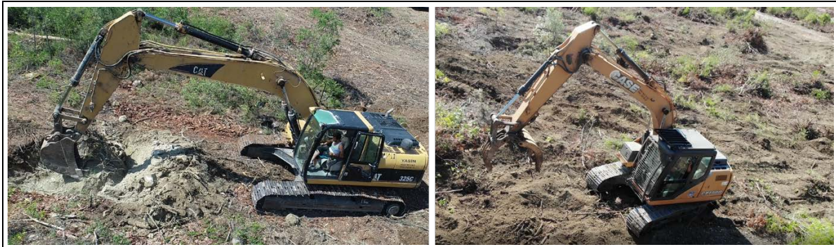
Figure 6. Excavator attachments for stump harvest: Bucket (at left) and Grapple Rake (at right)
