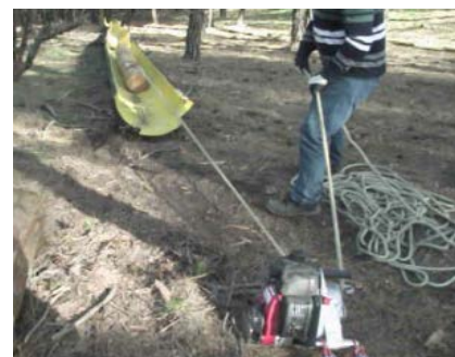
Figure 4. Chute system integrated with winch
