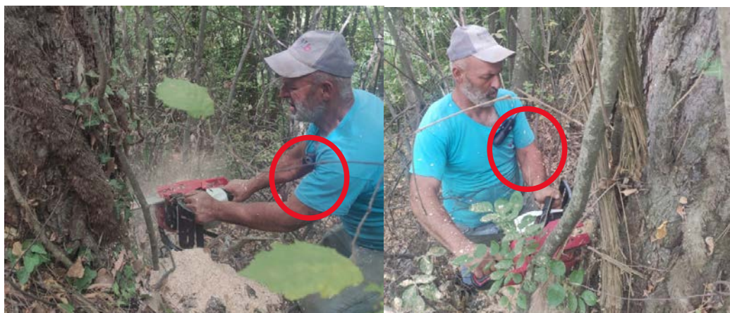
Figure 3. PM10 measurement in operator's breathing zone
