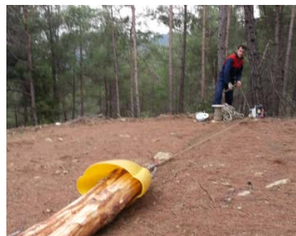
Figure 2. Cable pulling with a portable winch
