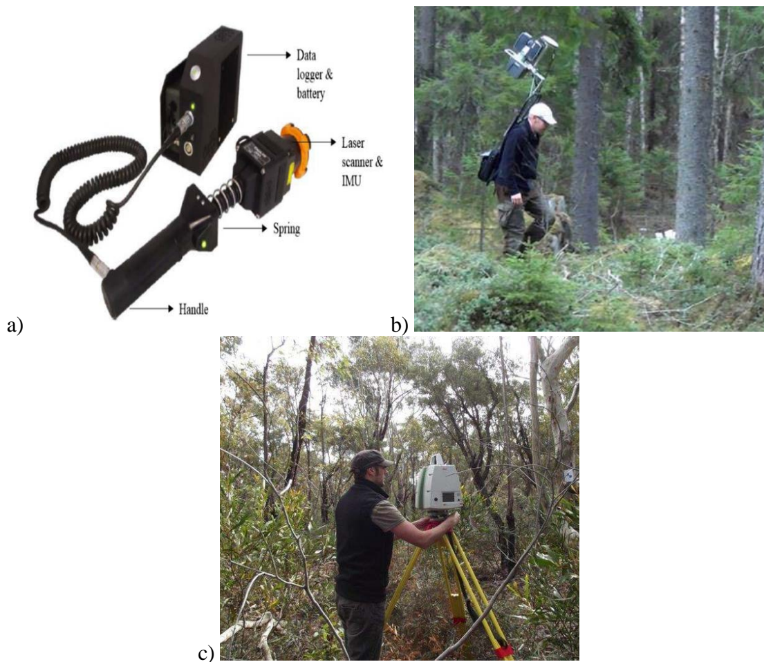
Figure 1. Handheld (a), backpack (b) and terrestrial (c) scanners (Shaw, 2022)
