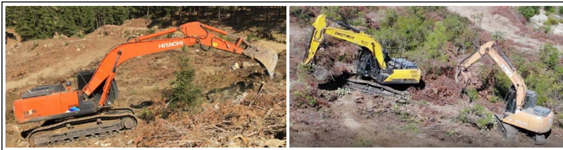
Figure 8. Excavator based stump harvest operations with different attachments
