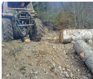
Figure 1. Cable pulling with agricultural tractor
