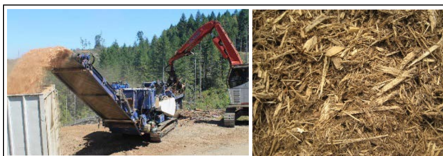
Figure 13. Grinding process for slash (at left) and hog fuel (ground material) (at right)
