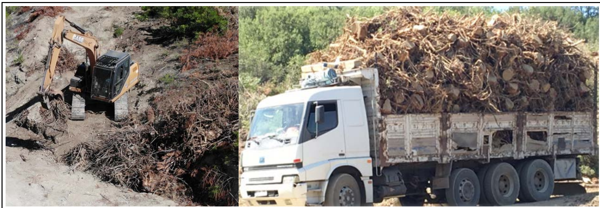
Figure 9. Sorting and loading of stump biomass with excavator and hauling with trucks
