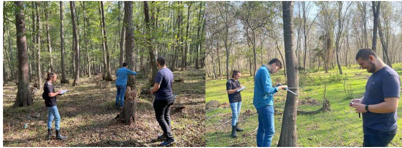
Figure 4. Traditional DBH and tree height measurement
