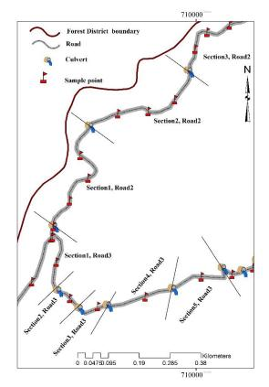
Figure 2. Dividing of road segments to sections based and culvert location in order to road inventory
