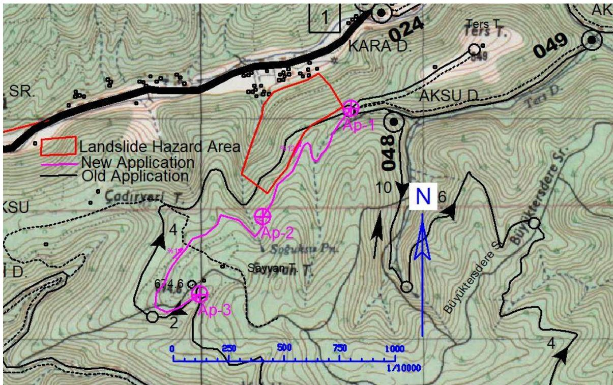
Figure 9. Road section within the landslide hazard area
