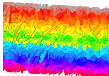
Figure 17.d. A request is entered for the density of the river network, in our case: value>5000. To implement this request, use the tool: Spatial Analyst- Conditional -CON with parameter: value>5000
