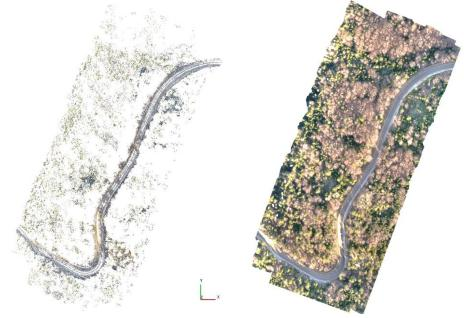
Figure 5. Tie points (left) collected during UAV flight and orthomosaic RGB image (right)
