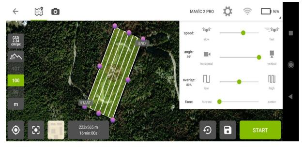
Figure 3. Flight area and settings on Pix4d interface
