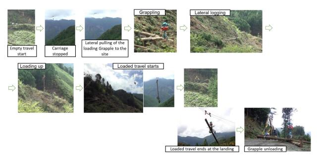
Figure 5. Sequence of the logging cycle
