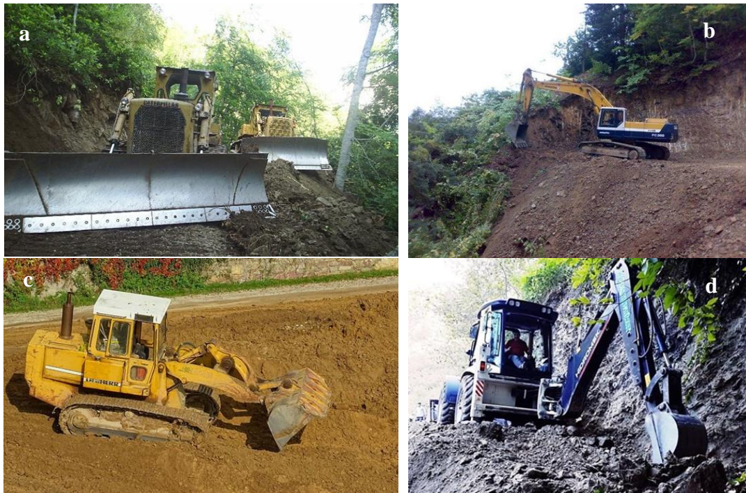
Figure 11. Forest road machines (a:Bulldozer, b:Excavator, c: Traxcavator, d:Backhoe)
