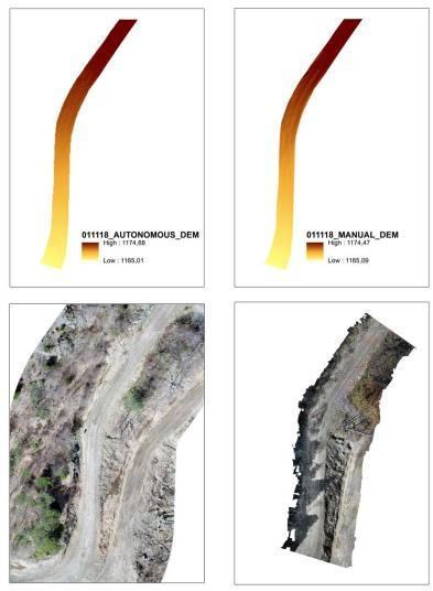
Figure 5. UAV based DEMs and orthophoto mosaics generated with manual and autonomous flights (01.11.2018)
