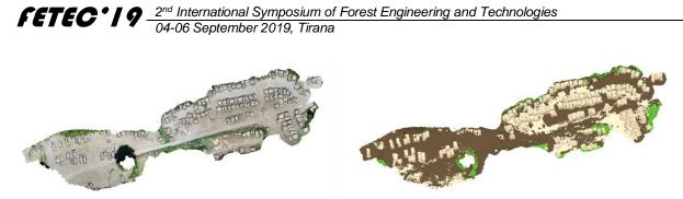
Figure 2. Dense point cloud (left) and dense point cloud classified into three classes such as ground (brown), high-vegetation (green), and man-made (corresponding to timber stowage) (white) (right)
