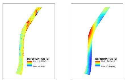
Figure 6. Deformation maps generated by both autonomous (left) and manual (right) flights
