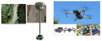
Figure 2. An example of GCP surveyed (left) and DJI Mavic Pro model UAV system (right)
