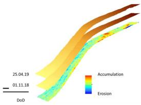
Figure 4. DoD (DEM of Difference) method applied to each two datasets
