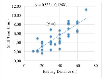
Figure 5. Plotting the relation between Pure Cycle Time (PCT) and cable hauling distance
