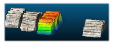
Figure 4. An example of stowage segmented and converted to the mesh
