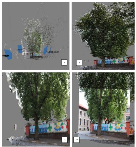
Figure 4. A) Tie points view of the tree with camera positions, B) Dense Point cloud view of the tree, C) 3D Model of the tree, and D) 3D Model overlay with the image of the tree.
