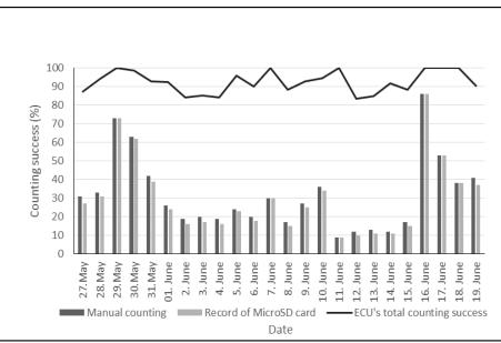
Fig. 2. Counting success rates with beetles counts determined manually and recorded by ECU
