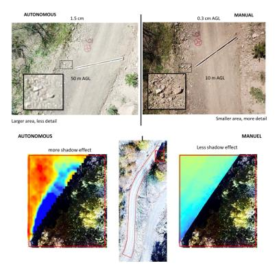
Figure 8. Comparison of autonomous and manual flights in terms of shadow effect (bottom) and object details in the images
