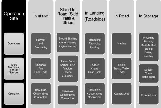
Figure 3. Traditional wood flow from stand to storage - Processes, inputs and actors
