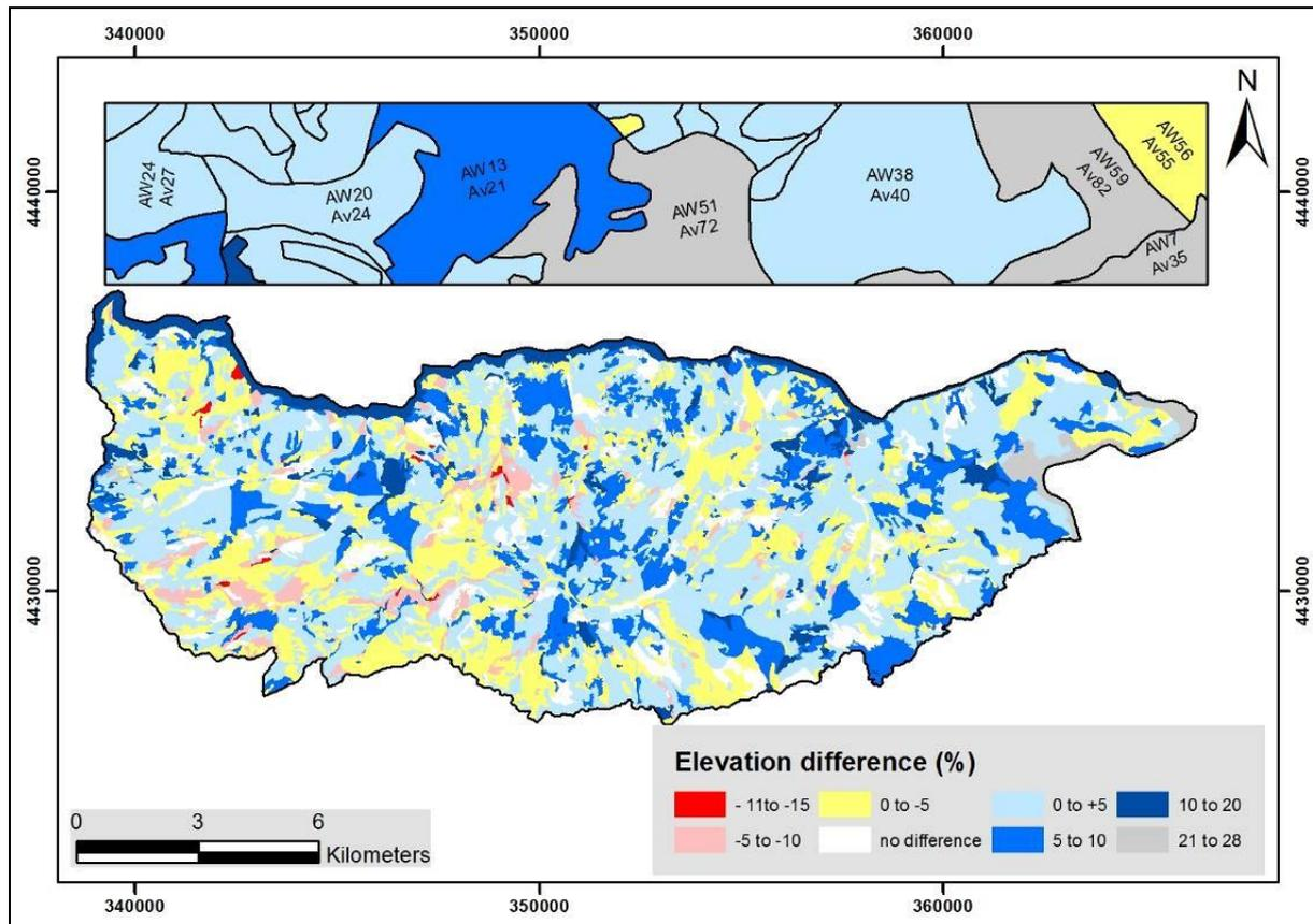
Figure 6. Slope deviation maps of Kızıltepe FPU (AW, Area weighted; Av, Arithmetic)
