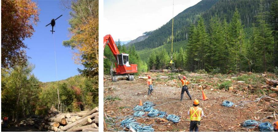
Figure 4. Placing logs on the ground (left) and releasing the lifting cable for next cycle (right)
