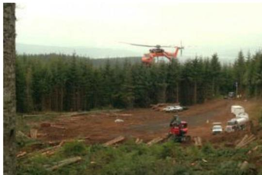
Figure 2. A logging helicopter flying inhaul from landing to harvest area
