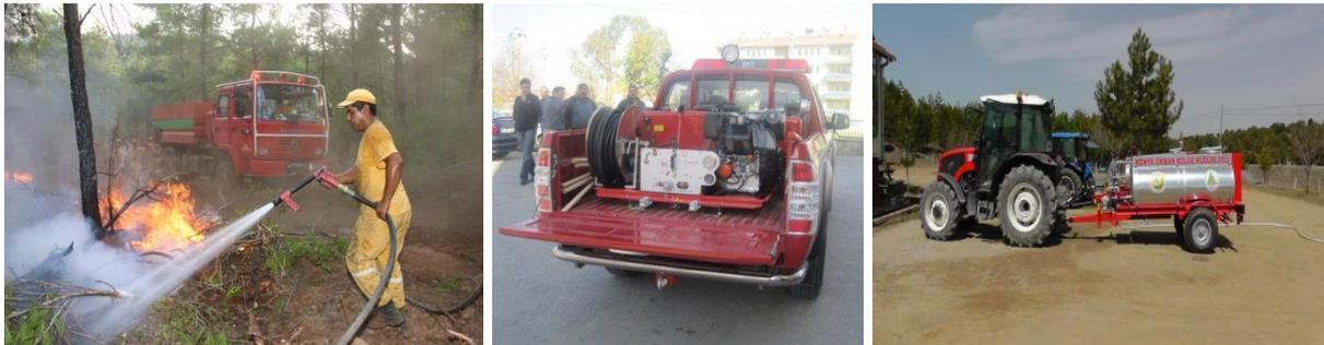
Figure 7. Sprinkler truck , First Responder Vehicle and Fire Extinguisher Tank
