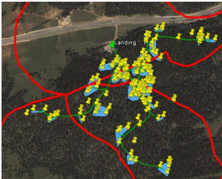
Figure 3. Point cloud of the fallen tree locations (yellow), distribution over four compartments (red), grouped trees (blue), skidding road route (green) and landing
