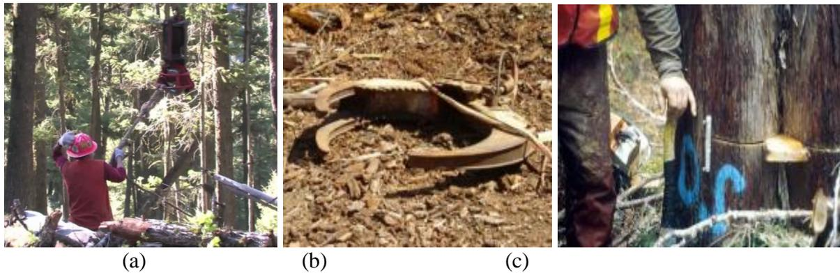
Figure 3. The hooker attaching chokers to the lifting cable (a), helicopter grapple (b), cut up standing stem (c)
