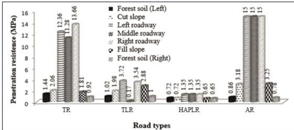
Figure 3. Penetration values according to road types
