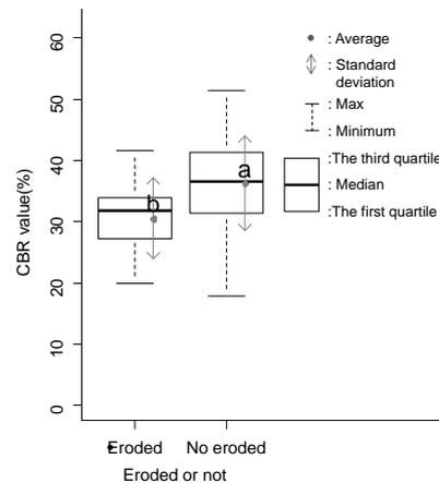
Figure 11. Relationships of CBR values between eroded and not eroded (Takahashi *et al.* 2015b) (Note: There is 5 % significant difference between “a” and “b”)
